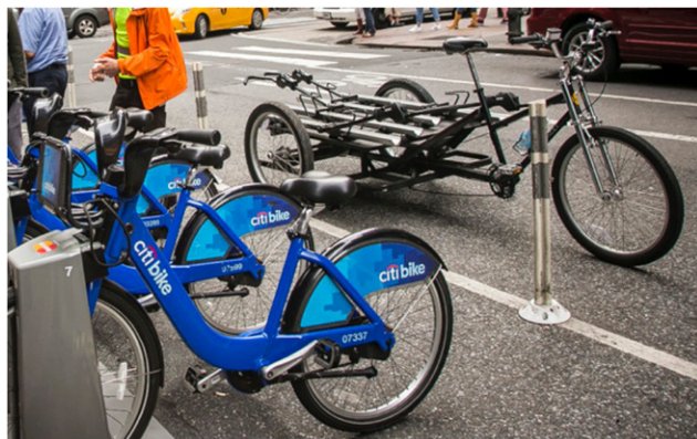
Figure 12. The Picture Shows a Trike that Citi Bike Uses to Transport up to Five Bikes in New York City
