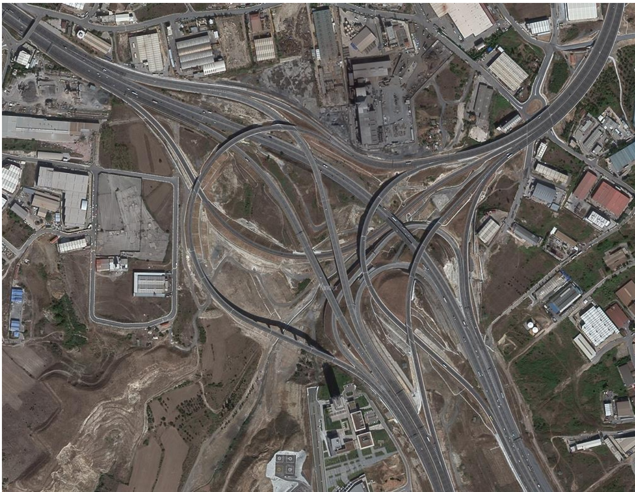
O-4, O-5 and O-7 junction in Kocaeli All-directional four-leg (or stacked interchange) (or spaghetti junction)
