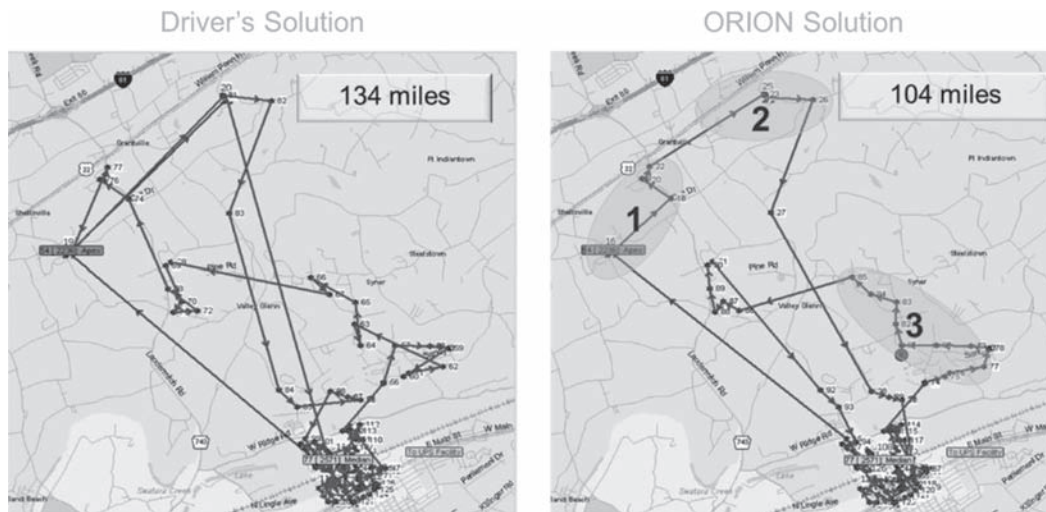
Figure 4. The driver on the route determined by ORION delivers in the shaded areas (Areas 1 and 2) only once; the driver-determined route does so twice. Both the driver and ORION visit Area 3 once, but ORION does so more efficiently. In this example, the ORION solution results in 30 fewer miles traveled while retaining some consistency with the base route.
